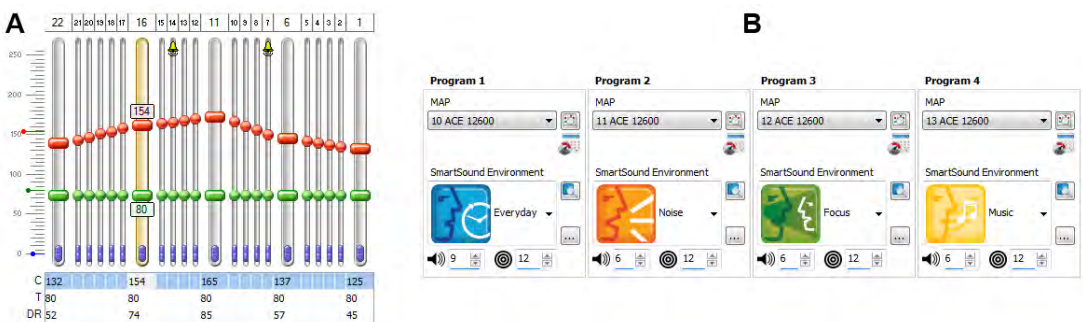
Figure 40: Screenshots of Cochlear's Custom Sound 4.0 fitting software. A: the default programming approach involves setting levels for only 5 electrodes out of 22 and interpolating those levels to the electrodes in between. B: programming of maps into the 4 available slots, each for a specific listening situation.
