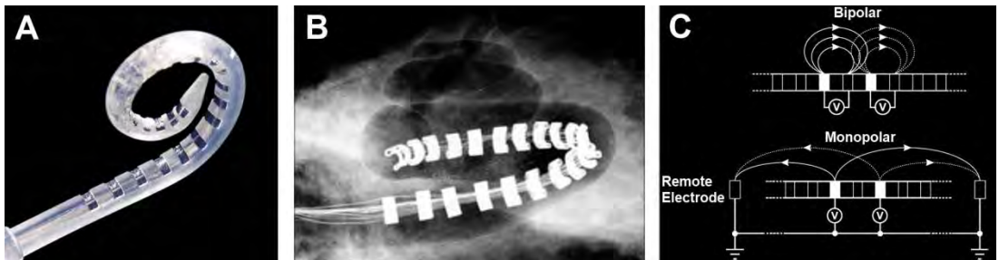
Figure 31: A: a cochlear implant electrode array (Cochlear's Nucleus Contour electrode). Its shape is precurved to minimize damage to cochlear structures and tissues during insertion. In addition, this type of perimodiolar (or "modiolus hugging") electrode minimizes the distance between electrode contacts and spiral ganglion cells that are target for stimulation. B: a phase-contrast X-ray image of Cochlear's Nucleus Contour electrode, a perimodiolar banded precurved electrode array, inserted into a cochlea. C: schematic of bipolar and monopolar electrode coupling. Solid lines indicate current paths of the actual stimulation cycle (time slice). Dotted lines represent a next time slice (assuming a sequential stimulation strategy). In bipolar stimulation mode a current circuit is established between the stimulating electrode and one of its neighbours, resulting in a locally constrained current flow. In monopolar modes, current flows from the actual stimulation contact to the extracochlear electrode(s). [A adapted from cochlear Ltd., B from Xu J et al., C from Clark GM]
