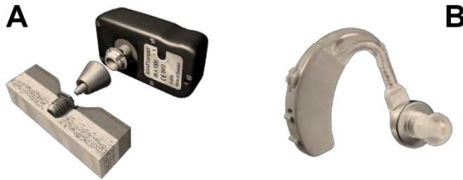
Figure 26: A: a bone anchored hearing aid, a semi-implantable percutaneous bone conduction hearing device coupled to the skull by an osseointegrated titanium fixture. The system transfers sound to the inner ear through the bone, thereby bypassing problems in the outer or middle ear. B: a conventional acoustical hearing aid, which amplifies sound before it is delivered to the eardrum. It has limited benefit for severe and profound sensorineural hearing losses, since it does not improve the frequency selectivity of the impaired inner ear. [A from Entific Medical Systems, B from Senlan Electronic Factory]
