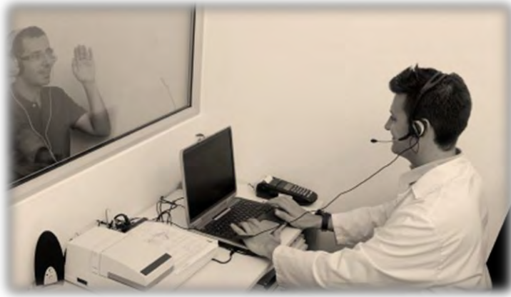
Figure 67: a typical setup for conducting psychoacoustical measurements, consisting of a calibrated audiometer to generate stimuli and/or control their presentation level, calibrated transducers (e.g. headphones or loudspeakers), a sound treated room to exclude interfering ambient noises and a computer operated by the examiner to execute the test protocol. [adapted from Banús CM]
