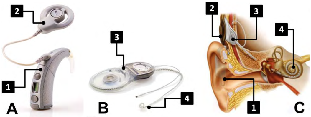
Figure 29: The main parts of a cochlear implant. Its external parts (A) are a speech processor (1) that can be worn behind the ear and a transmitter coil (2). Internally (B) there is a receiver-stimulator (3) and the electrode array (4) positioned in the inner ear (C). [A,B adapted from Cochlear Ltd., C from sacic.com.au ]
